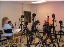
Figure 3. VICON motion capture system with 8 cameras. The subject with the markers sat in the middle of the room, with the cameras directed to him/her. The subject without the markers sat outside the field of view of the VICON cameras, facing the subject with markers.
